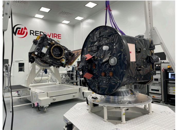
— Proba-3 Occulter and Coronagraph spacecraft
