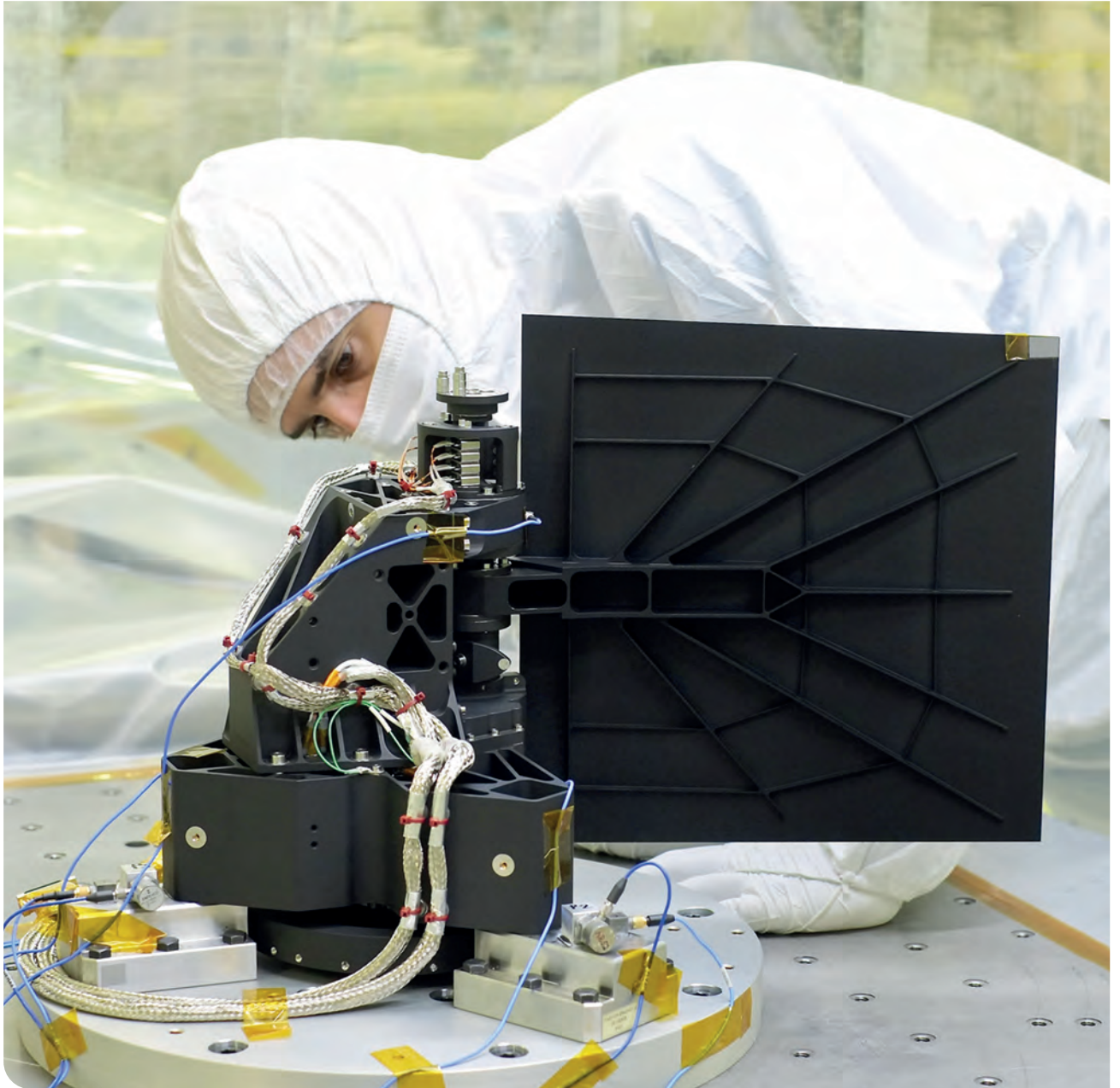
The VIS Read-Out Shutter Unit (RSU) mechanism for Euclid from APCO Technologies. Image credit: APCO.
