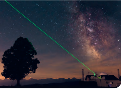
Laser beam transmitted from the 1-meter ZIMLAT telescope to measure mm-accuracy distances of artificial satellites.
