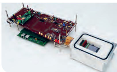
Front-End Electronics during characterisation.
