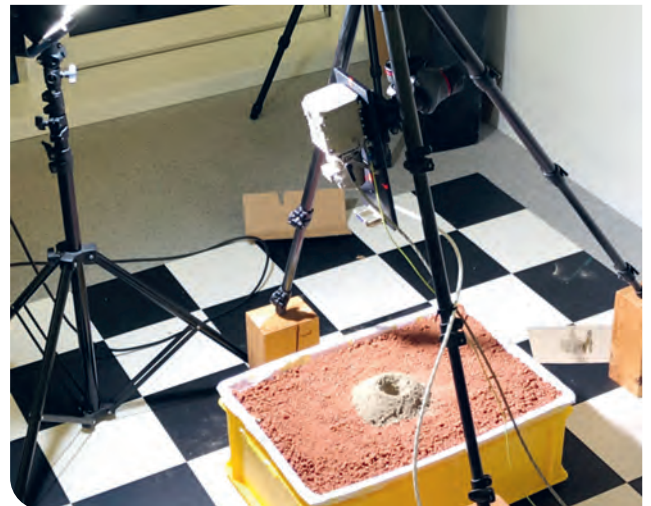
Top left: CAD view of CLUPI taking images of the sample in the drawer of the rover. Bottom left: CAD view of CLUPI taking images of the hole and drill fines. Top and bottom right: CLUPI Flight Model Representative on a Drill/Rover simulator taking pictures of samples and of a hole with drill fines during operations simulations in the CLUPI Science Operations Lab. of SEI in Microcity (Neuchâtel, Switzerland). Image credits: SEI.
