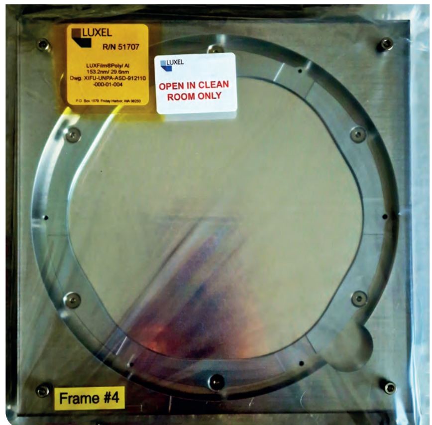
One of the four full-scale X-IFU optical blocking filters procured by the UNIGE team from LUXEL (USA). The filter membrane is mounted on an aluminum frame, designed and manufactured by UNIGE. The filter has a clear aperture of 160 mm, and the photo shows the complex honeycomb structure of the metallic mesh, glued on the filter to support the membrane.
