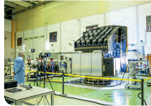
The Plato STM with its 26 telescopes (24 + 2) on the QUAD shaker at ESA/ESTEC. The Spacecraft is undergoing vibration tests to simulate launch conditions.
