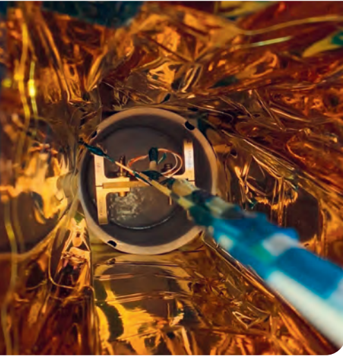
Picture taken during the thermal cycling test of the SXI support assembly breadboard to verify the durability of the selected materials (fibre-reinforced plastic and aluminum) at ZHAW. Image credit: ZHAW.
