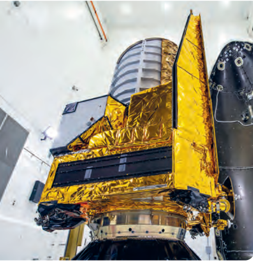
Euclid moments before it was encapsulated in a SpaceX Falcon 9 fairing. Image credits: SpaceX/ESA.
