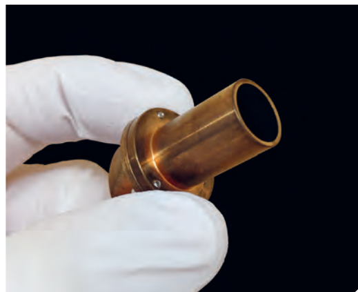
A prototype sensor cavity for the Cryogenic Solar Absolute Radiometer (CSAR).
