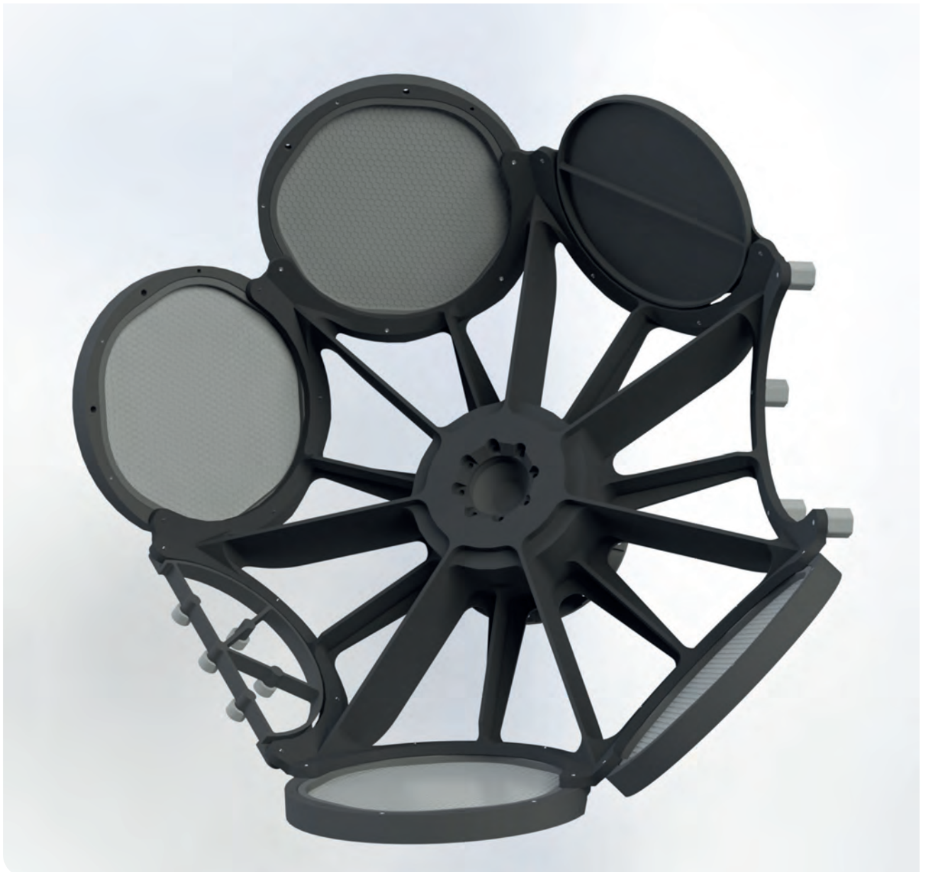
Sketch of the present University of Geneva preliminary design for the LEM filter wheel. The wheel hosts four positions for different filters, plus an open position, a closed position, and a position to place the required radioactive ^{55}\text{Fe} calibration sources.
