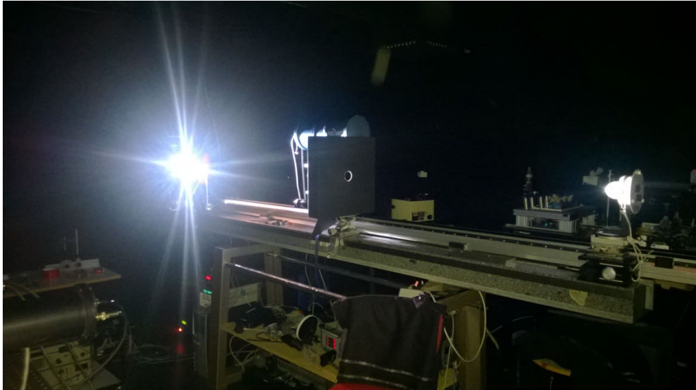
Figure 9. Angular response setup of the WCC-UV.
