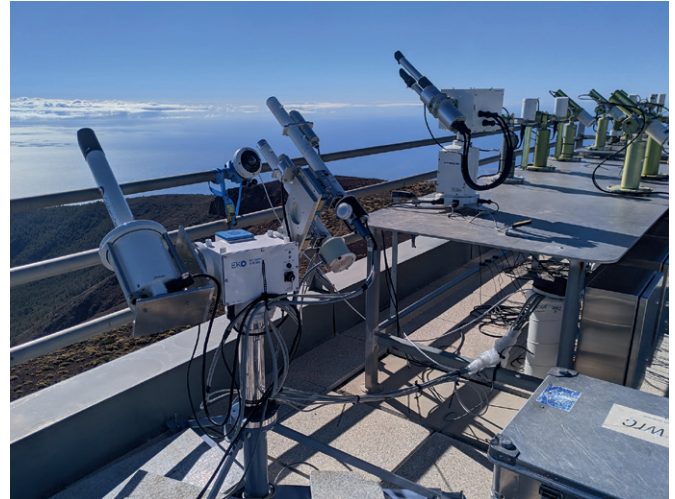
Figure 2. EMPIR MAPP campaign at Izaña (Spain) with the Qasume and QasumeIR spectroradiometers in the centre of the picture.
