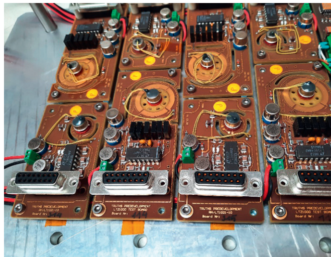
Figure 4. Voltage references mounted on a test jig used in a proton irradiation test.
