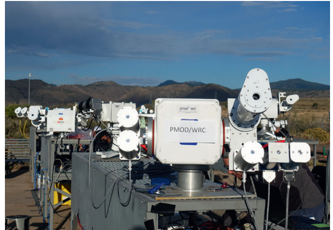
Figure 1. The WRC-SRS travelling standard group against the backdrop of the Rocky Mountains at the National Pyrheliometer Comparison (NPC) in Golden, USA. The travelling standard group consists of the four absolute cavity radiometers mounted on the right-hand side of the solar tracker. The radiometers on the left belonged to Davos Instruments AG.
