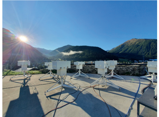
Figure 2. Brewer instruments during the 2022 Regional Brewer Calibration Campaign for Europe (RBCC-E) in the measurement field at PMOD/WRC with the participation of the World Brewer reference from Toronto (Canada).
