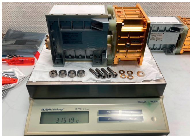
Figure 1. Physical properties (mass) verification of the DARA Flight Spare model.
