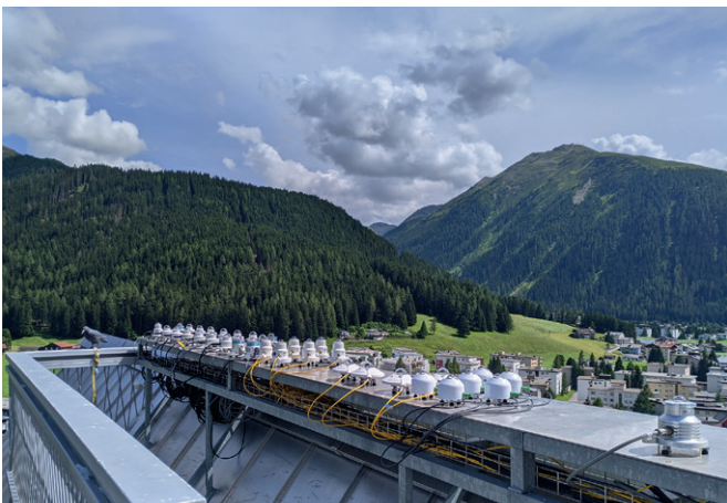
Figure 1. The UVC-III campaign at PMOD/WRC lasted from June to August 2022. UV radiometers from the campaign are seen in the above picture on the roof platform.
