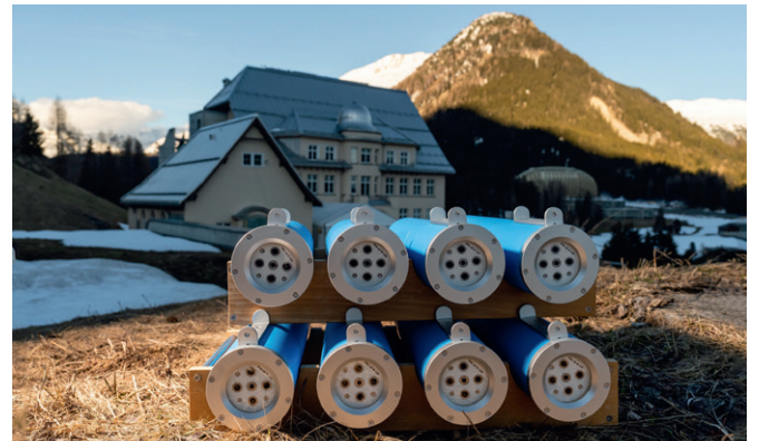
Thirty Precision Filter Radiometers (above) and five new IRIS radiometers (below) were built.
