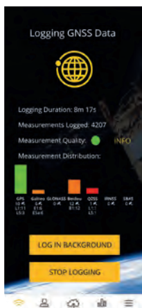
Screenshot from the Camalot Android app that allows users to collect and share raw GNSS data.
