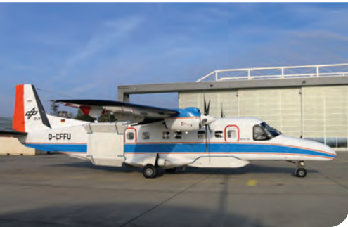
DLR's F-SAR sensor on the Dornier DO 228 carrier platform: The antenna system is mounted at the rear of the aircraft. Image credit: DLR.
