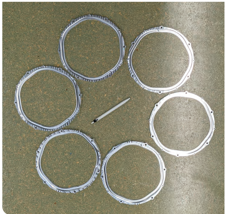
X-IFU filter wheel filter frame prototypes manufactured by UNIGE. The layout around a typical Swiss-made Caran d'Ache ballpoint pen shows the approximate size of the mechanism hosting in total seven positions. The filters have a clear aperture of 160 mm.
