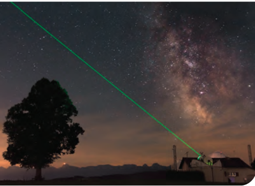
Laser beam transmitted from the 1-meter ZIMLAT telescope to measure the distances of artificial satellites with a mm-accuracy.
