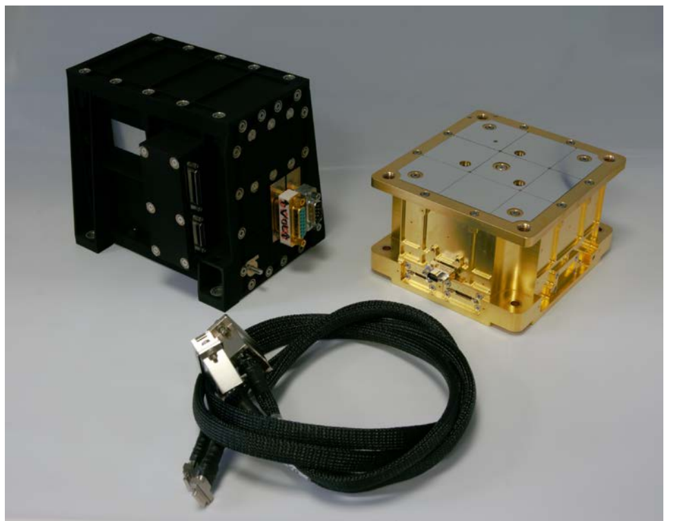
DARA measurement unit (gold), control unit (schwarz) and cables.
