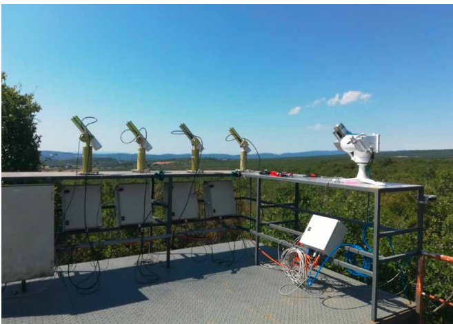
Figure 1. Platform at the Observatoire de Haute Provence (OHP), France with four CIMEL sunphotometers and the travelling standard PFR on its own solar tracker (right).
