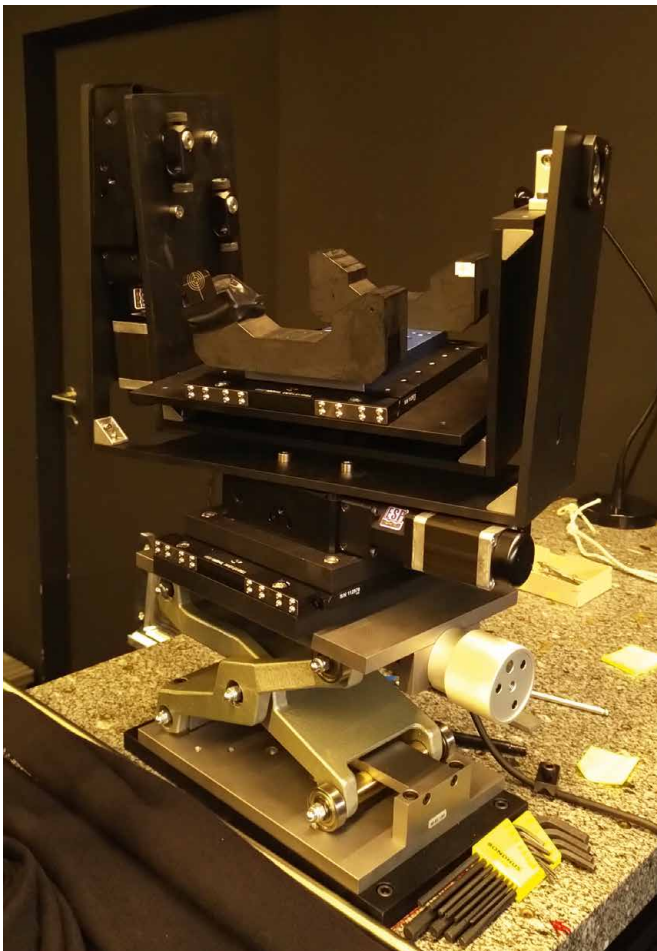
Figure 1. The new Angular Response Function (ARF) pointing measurement setup of the WRC with two Newport goniometers.
