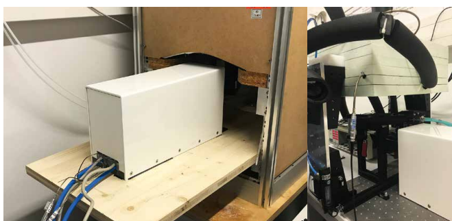
Figure 1. Left panel: TSRT placed below the aperture of the PMOD/WRC blackbody. Right panel: TSRT placed below the aperture of the HSBB. A gold-plated mirror connected to the TSRT reflects the radiation emitted by the cavities to the TSRT.
