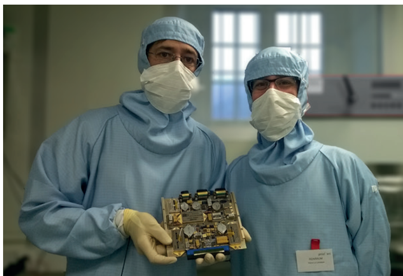
FM of the LVPS for the SPICE instrument, built at PMOD/WRC by Daniel Pfiffner (left) and Pierre-Luc Lévesque (right), was delivered to RAL for inspection and afterwards to SwRI for integration into the SPICE FM electronics box.
