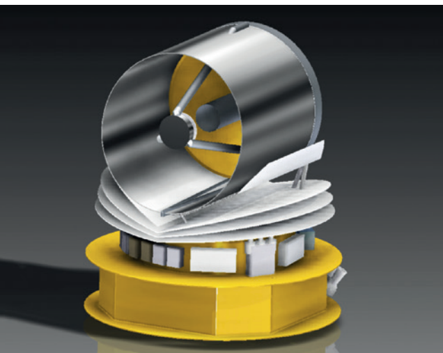
The SPICA satellite (Planck configuration, 2.5m@8K telescope).
