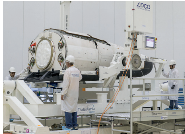
Preparation of the Intermediate eXperimental Vehicle (IXV), APCO Technologies—Mechanical Ground Support Equipment.
