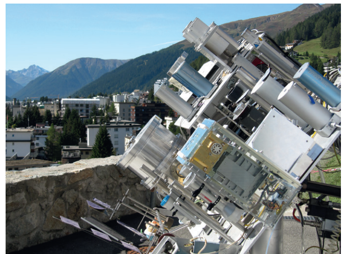
Figure 3. DARA EQM/FS mounted on the WRC main solar tracker.
