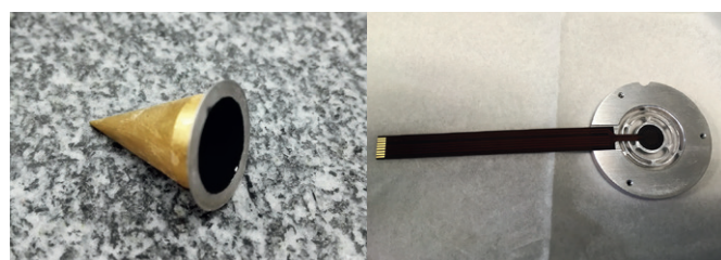
Figure 1. Left panel: Old cavity installed in previous radiometers. Right panel: the new flat receiver.
