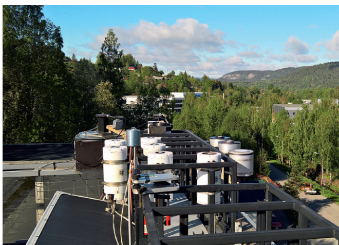
Figure 1. The DSA station in Oslo, Norway, showing the QASUME entrance optics (dome with blue cylinder) towards the front of the platform, while the GUV and NILU radiometers, and the local spectroradiometers are at the far end.
