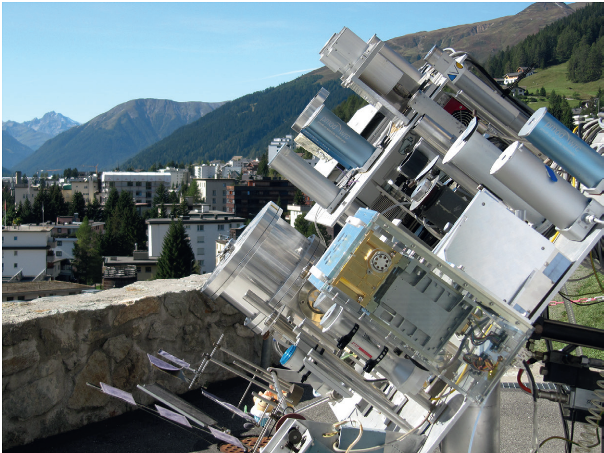
Figure 3. The Digital Absolute Radiometer (DARA), designed and constructed at PMOD/WRC, is a payload onboard the ESA PROBA-3 satellite mission, which will be launched in the near future. The picture shows the DARA EQM/FS (Engineering Qualification Model/Flight Spare) in the foreground (center right), mounted on the WRC main solar tracker during calibration at PMOD/WRC.
