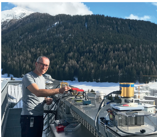
Figure 4. Installation of the NREL ACP (foreground) and three IRIS radiometers on the PMOD/WRC measurement platform by C. Thomann.
