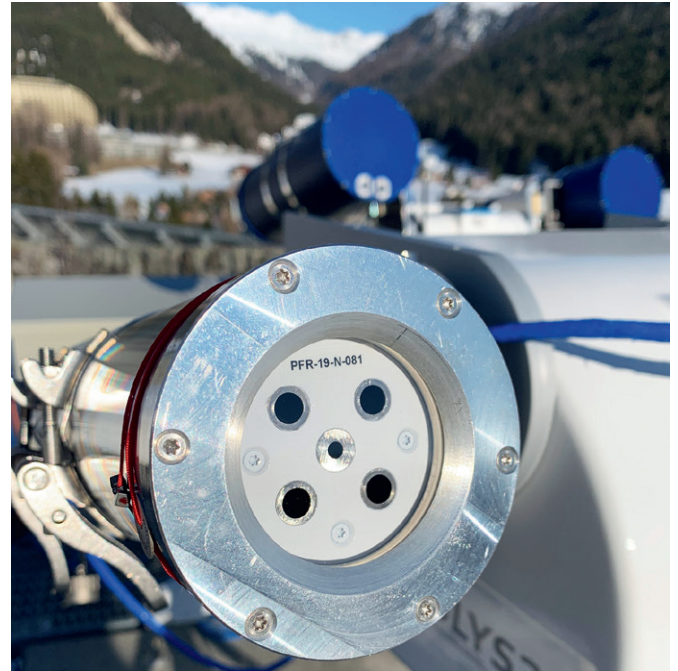
Figure 1. The new Precision Filter Radiometer (PFR) series, along with two Precision Spectroradiometers in the background.
