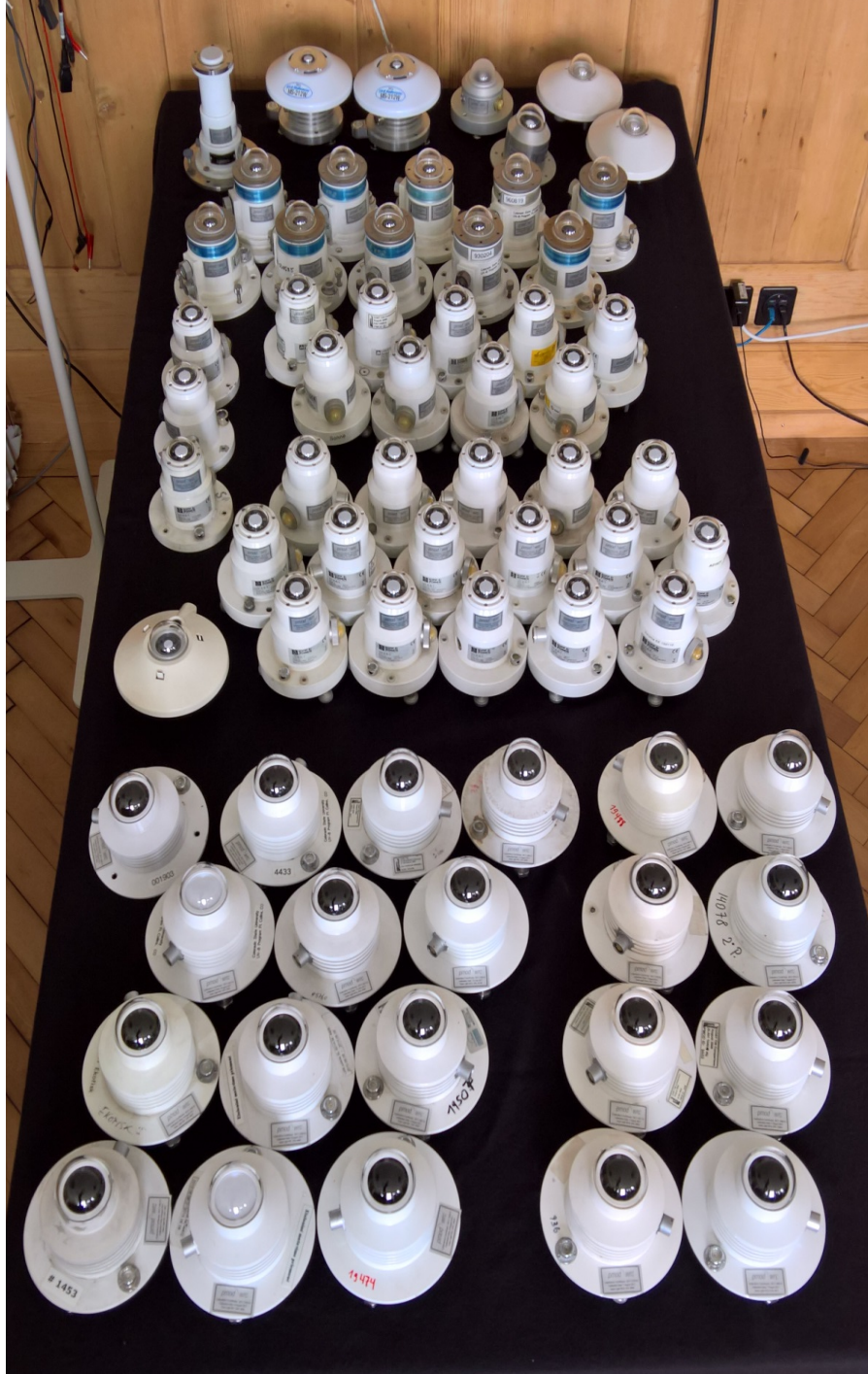
Figure 6. Picture of the main set of participating radiometers. SL (front), KZ/Sintec (middle), YES (back), Delta Ohm, Indium Sensor, Genicom, Eppley, EKO and Middleton Solar (last row).
