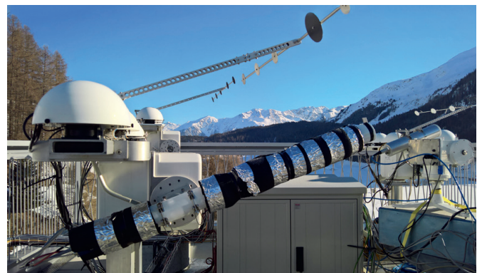
Figure 3. The QASUME portable reference spectroradiometer measuring direct irradiance on the PMOD/WRC roof. The input optic is at the end of the 940 mm long collimator tube.
