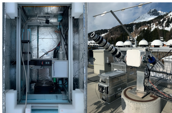
Figure 1. Left) temperature-stabilised housing of the KOHERENT system. Right) outdoor operation (KOHERENT telescope on the right of the solar tracker and QASUME telescope on the left).
