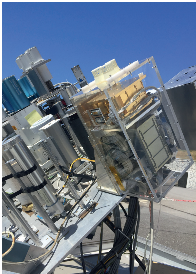
Figure 6. DARA radiometer for the JTSIM PFM instrument (inside the perspex box) installed on the World Standard Group (WSG) tracker during first solar measurements.
