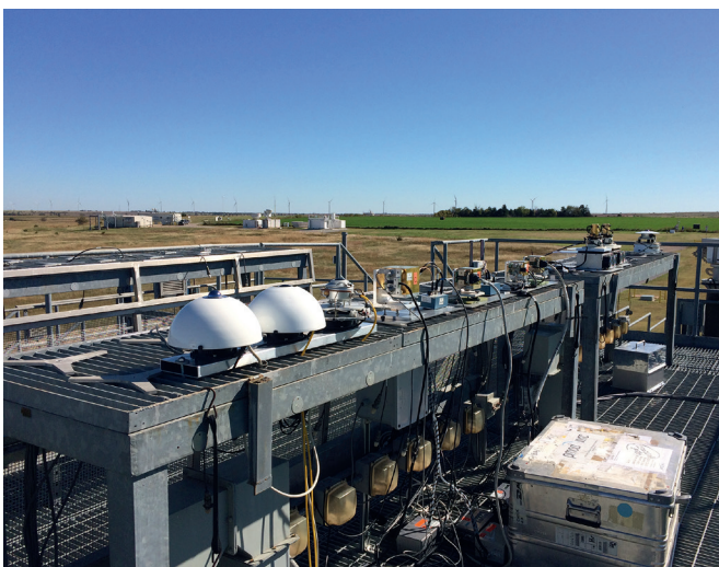
Figure 4. Radiometers to measure downwelling longwave radiation during the inter-laboratory comparisons at the SGP site in Oklahoma, USA.
