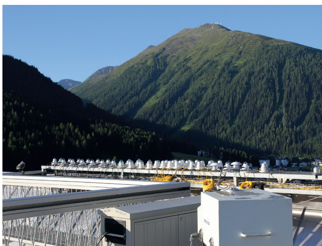
Figure 1. Outdoor calibration during the 2 nd International UV Filter Radiometer Comparison (UVC-II) on the PMOD/WRC roof platform with a total of 75 UV radiometers.
