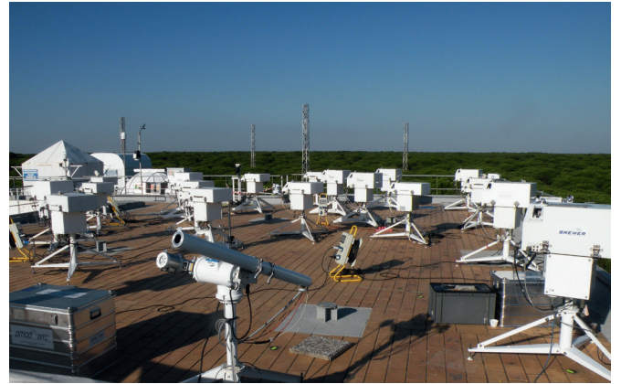
Figure 2. View of the measurement platform at the Instituto Nacional de Technica Aeroespacial (INTA). The input optic for direct irradiance measurement of QASUME can be seen at the front of the image.
