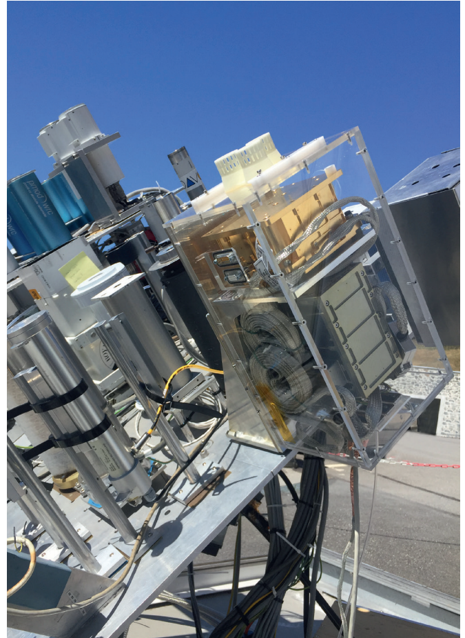
Figure 8. JTSIM-DARA being calibrated against the World Standard Group at PMOD/WRC.
