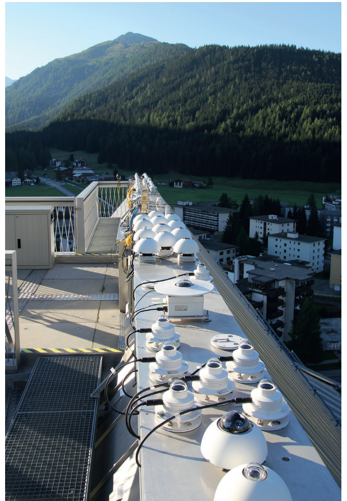
Figure 3. Outdoor calibration during the 2 nd International UV Filter Radiometer Comparison on the PMOD/WRC roof platform with a total of 75 UV radiometers.
