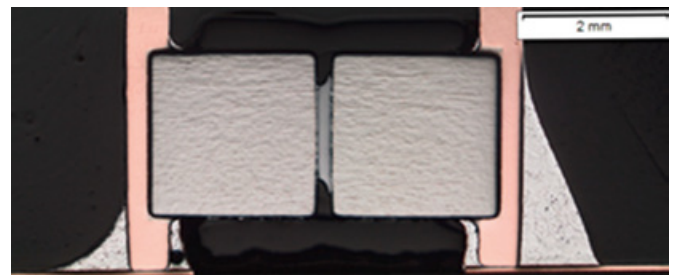
Figure 2. Micrograph of a component from the solder verification board.
