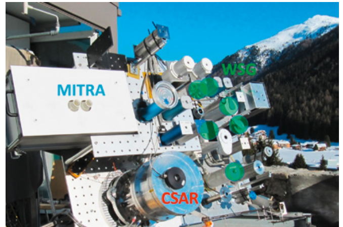
Figure 1. The CSAR and MITRA instruments next to the WSG on the sun tracking platform at PMOD/WRC measuring direct normal solar irradiance.
