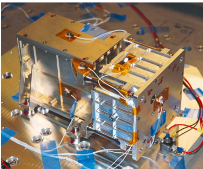
Figure 7. DARA Engineering Model on a vibration adapter during testing.
