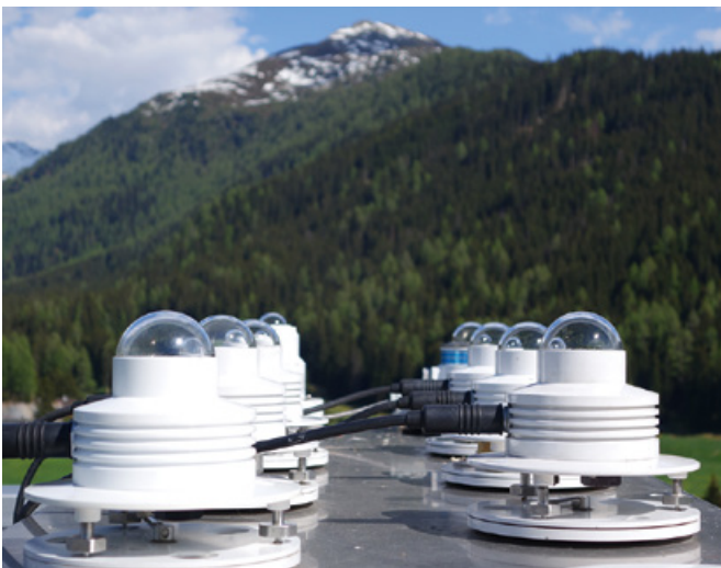
Figure 4. Calibration of Customer UV broadband radiometers.
