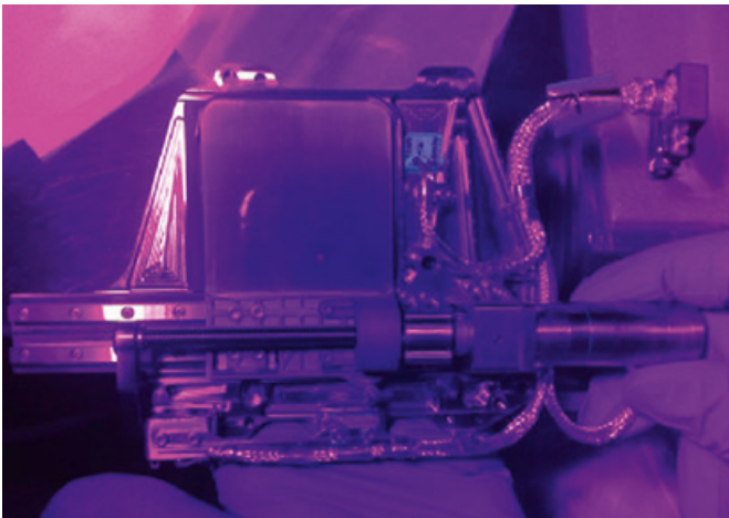
Figure 4. Inspection of the SPICE Door Mechanism (SDM) Flight Model under UV light during final assembly.
