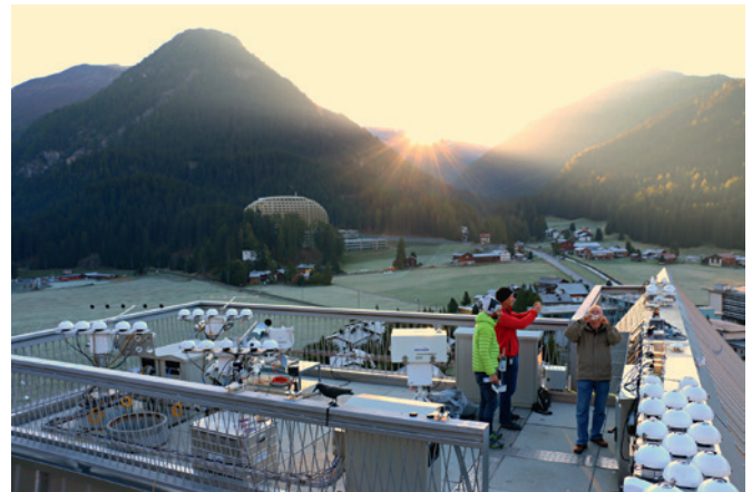
Figure 1. Roof platform of PMOD/WRC at sunrise during the pyrgeometer comparison. The WISG pyrgeometers are mounted on the far left-hand solar tracker, while the IRIS radiometers are on the unshaded roof platform, on the right-hand side.
