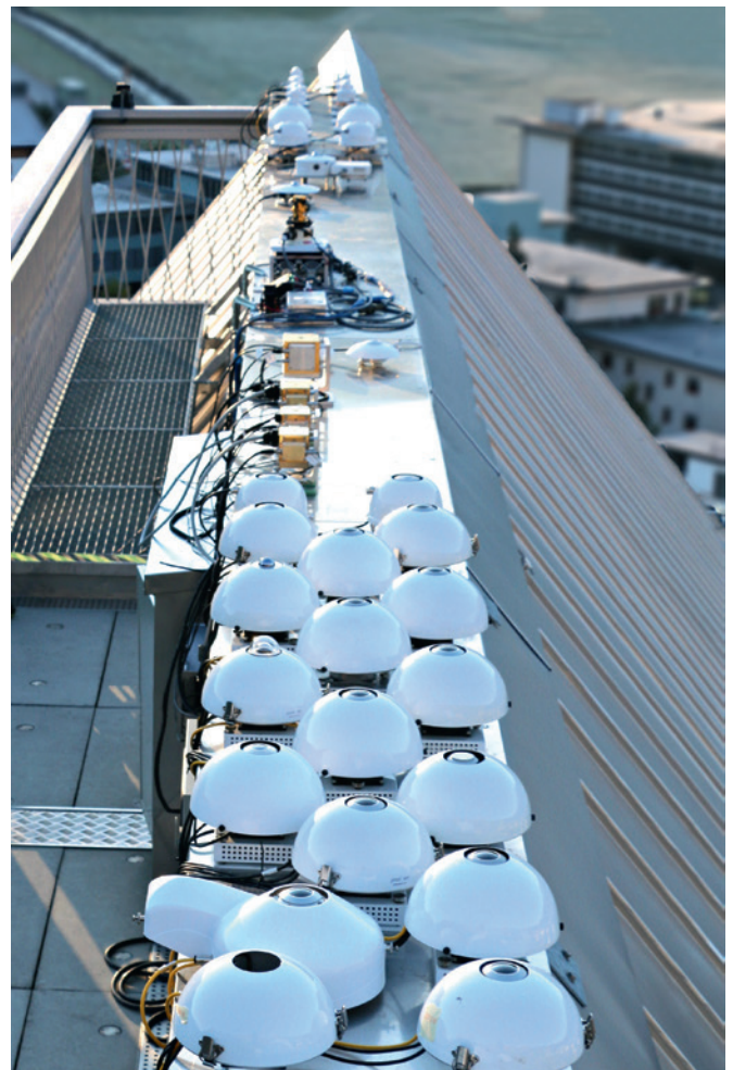
Figure 2. View of the PMOD/WRC roof-platform during IPgC-II, showing pyrometers in the foreground.
