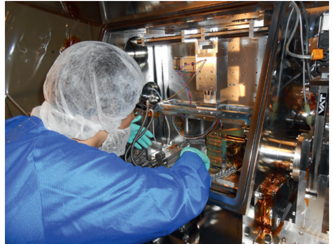
Figure 1. PMOD/WRC engineer Pierre-Luc Lévesque installing the CLARA radiometer in the TRF vacuum tank in Boulder, USA.
