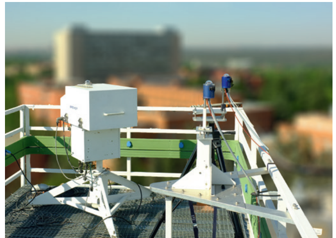
Figure 2. QASUME site audit in Madrid to assess the quality of the Brewer #186 spectrophotometer and the AEM Bentham DM300 double monochromator.
