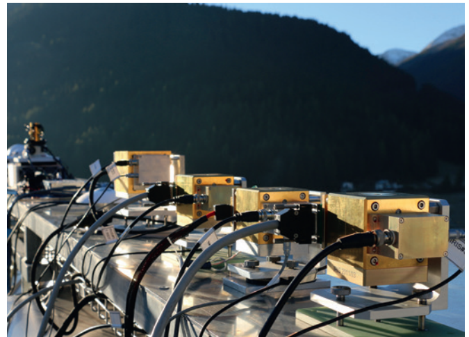
Figure 1. IRIS radiometers in operation on the PMOD/WRC roof platform during IPgC-II. The Absolute Cavity Pyrometer (ACP) from the National Renewable Energy Lab. (NREL; USA) can be seen on the left-hand side, at the back of the platform.
