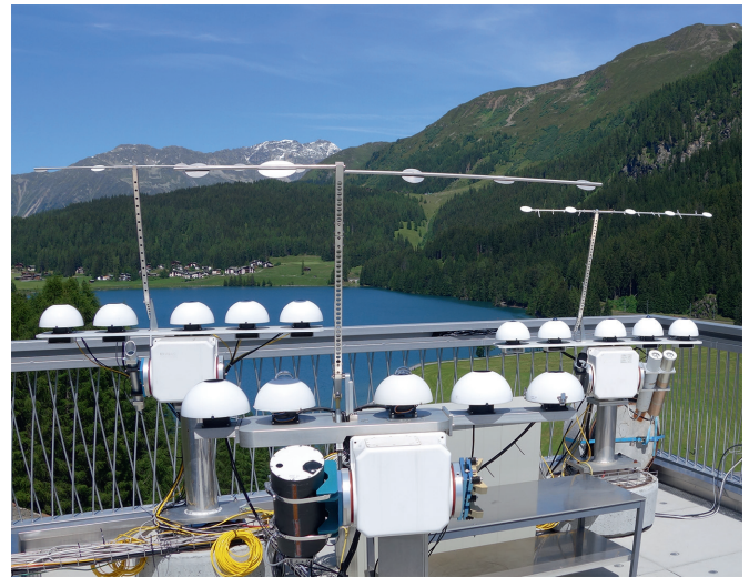
Figure 1. The WISG (far right) and other customer pyrgeometers on the PMOD/WRC roof-top with Lake Davos in the background.
