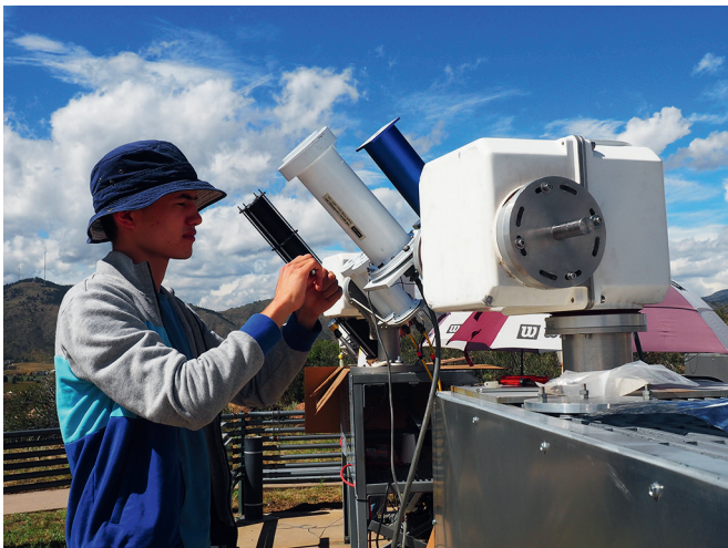
Figure 1. Nathan Mingard setting up the PMOD/WRC's transfer standard group to conduct solar irradiance measurements during the National Pyrheliometer Comparison at NREL in Golden, USA.
