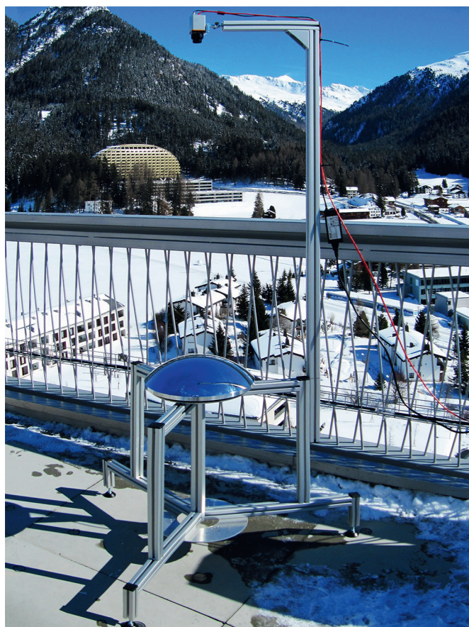
Figure 1. The InfraRed Cloud CAM (IRCCAM) on the PMOD/WRC roof in Davos, Switzerland
