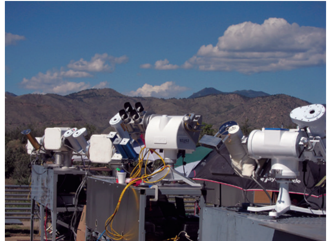
Figure 1. Pyrheliometers measuring the solar irradiance during the US National Pyrheliometer Comparison (NPC-2013) in front of the foothills of the Rocky Mountains in Golden, Colorado.
