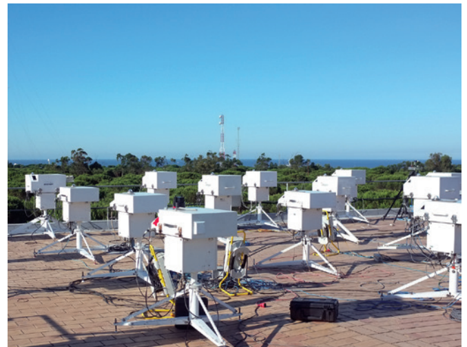
Figure 2. Brewer spectroradiometers during a calibration campaign at INTA, Spain.
