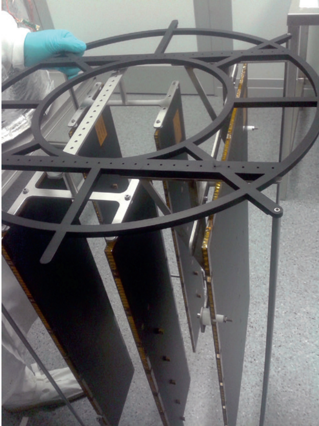
Figure 3. Panel bake-out preparations at PMOD/WRC which are conducted in a clean-room environment.
