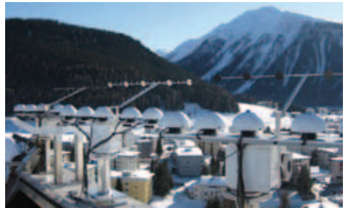
Figure 1. View of the measurement platform of WRC-IRS on the top of the PMOD observatory. The picture was taking facing South in January 2009. The solar tracker closest to the viewer hosts the World Infrared Standard Group (WISG) of pyrgeometers, while the other two are equipped with customer pyrgeometers.
