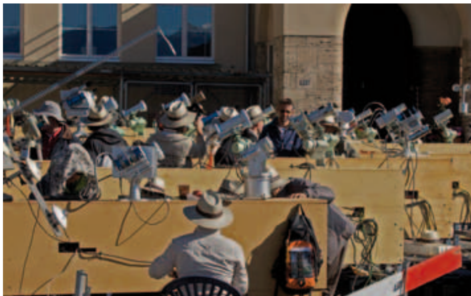
Figure 1. IPC-XI participants are concentrating on accurately pointing and timing their pyrheliometers. Solar irradiance levels depend strongly on atmospheric conditions. Accurate comparison of instrumental sensitivities are only possible with simultaneous irradiance measurements. Therefore scientists from all over the world gather at PMOD/WRC every five years to ensure compatibility of their solar irradiance data with the World Radiometric Reference (WRR). Photo: Ellen Røed, Norway.
