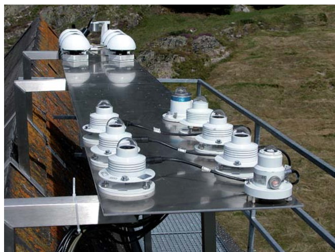
Figure 3. The roof-platform of PMOD/WRC showing the UV broadband radiometer reference triad among others.
