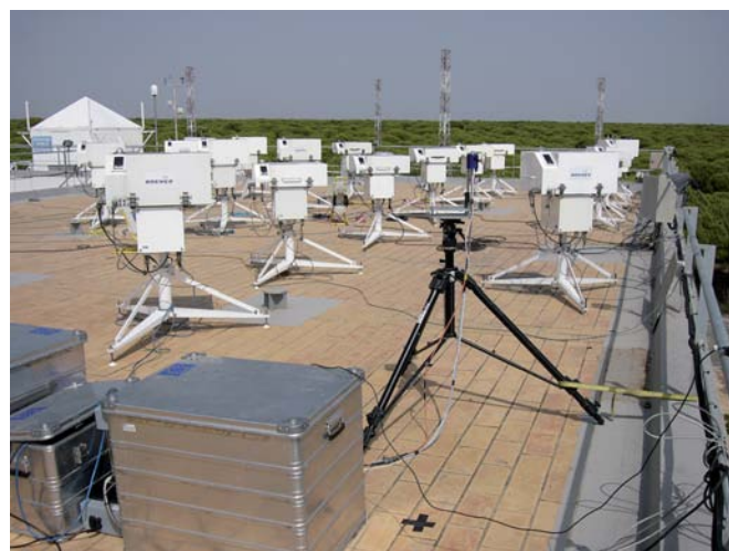
Figure 4. 2 nd RBCC-E campaign in El Arenosillo, Spain, with the transportable spectroradiometer QASUME acting as UV reference instrument.
