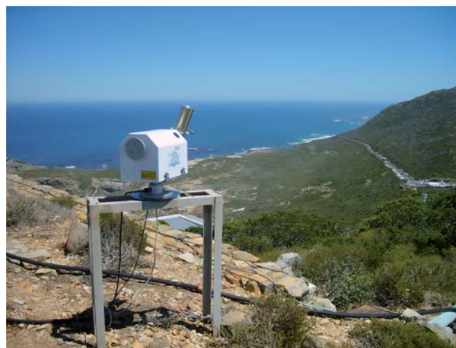
Figure 1: At Cape Point on the southern tip of Africa, a PFR has started observations of AOD.
