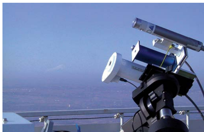
Figure 1: The WRC/SRS travelling standard with PMO5 (top), PMO6-0401 (middle) and AHF-32455 (bottom) during the WMO Regional Pyrheliometer Comparison of RA-II (Asia) on Mount Tsukuba, Japan. In the distance the snow-covered slopes of Mount Fuji are just visible.
