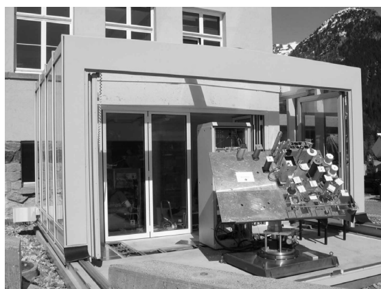
Figure 1 and 2. New glass-building that houses the World Standard Group. Left: Building closed. Right: The front part of the building has been moved back to expose the sun tracker and to enable solar measurements.
