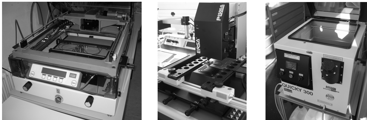
Figure 13. The new Surface Mount Technology equipment: solder paste printer (left), surface mounted devices repair-work station with micromanipulator (middle), and vapor phase reflow oven (right).
