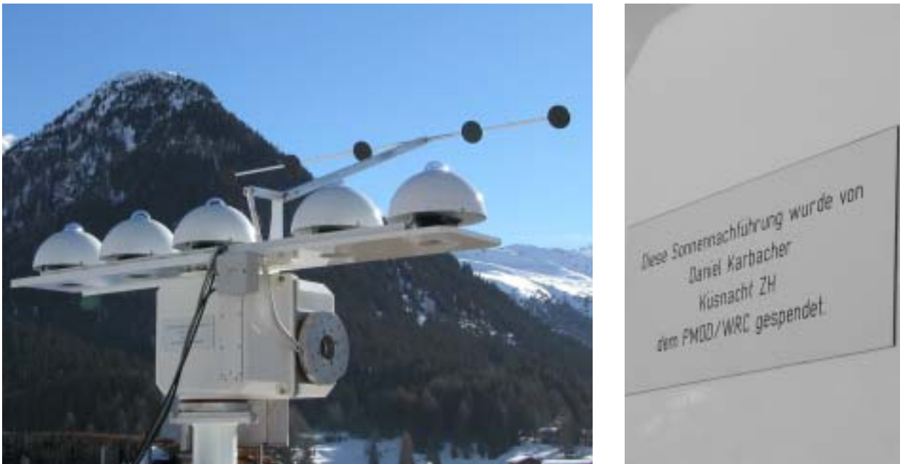
Figure 14. Sun tracker with sun shades shielding pyranometers from direct solar radiation. As the panel on the right side informs, this sun tracker was sponsored by Daniel Karbacher.
