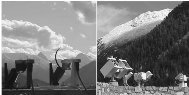
Figure 3. Some instruments participating in filter radiometer comparison (left plate: 2 rotating shadow band radiometers; right plate: 7 tracking radiometers) under examples of prevailing sky conditions.
