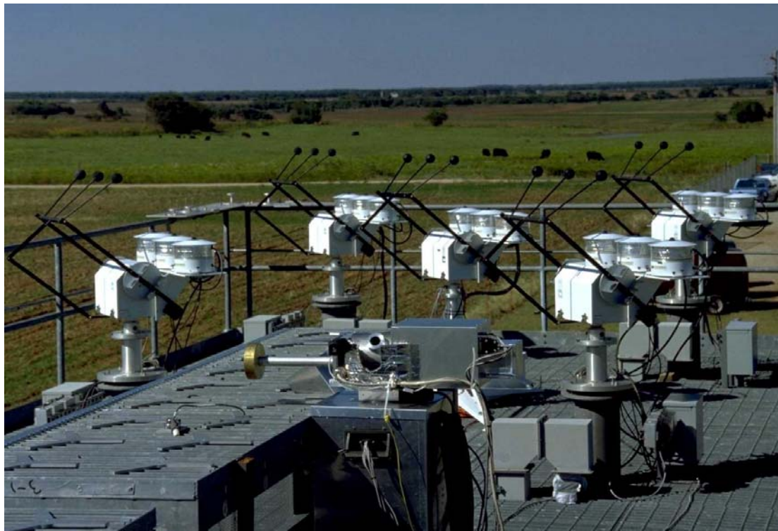
Figure 7: Pyrometers set up on solar trackers and PMOD/WRC absolute sky-scanning Planck Calibrated Sky Radiometer (PCSR) on the radiation trailer of the SGP-CART site at Oklahoma in September 1999.
