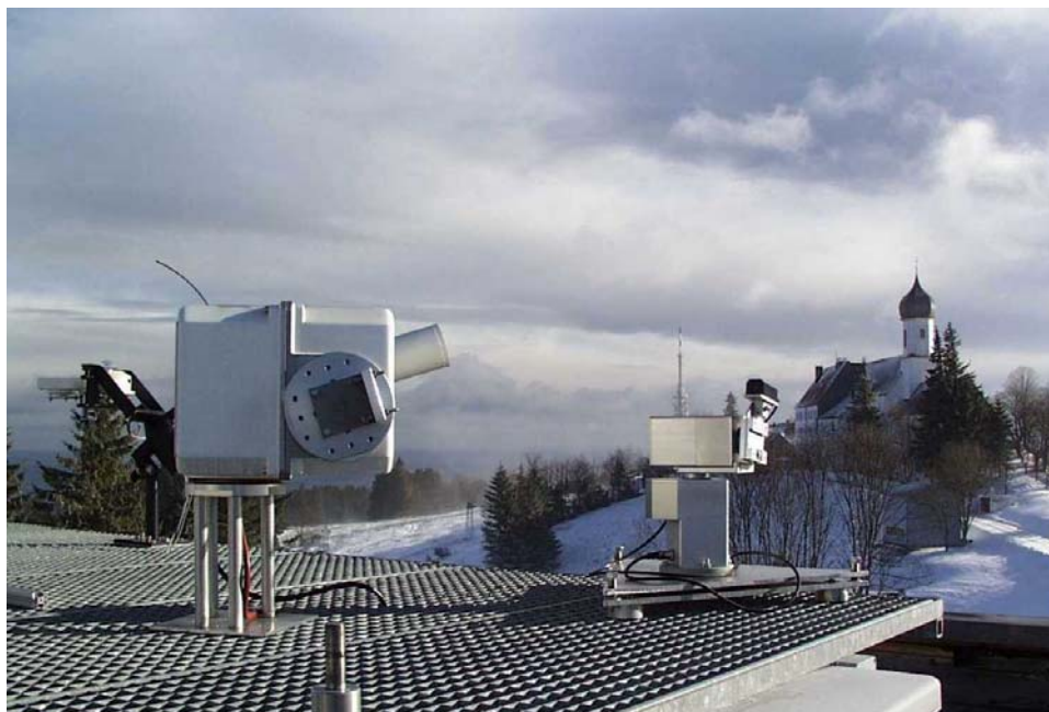
Figure 3: Precision Filter Radiometer PFR-N06 mounted on the roof platform at Hohenpeissenberg pointing at the Sun under less than favorable weather conditions.
