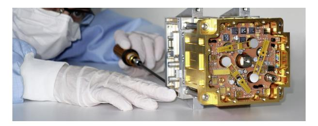
Picture. The Compact Lightweight Absolute Radiometer (CLARA), a payload on board the Norwegian NorSat-1 nano-satellite. CLARA is a new generation of radiometers to measure the Total Solar Irradiance which continues the long-term involvement of the PMOD/WRC in space and solar research. CLARA was funded by Swiss PRODEX.
