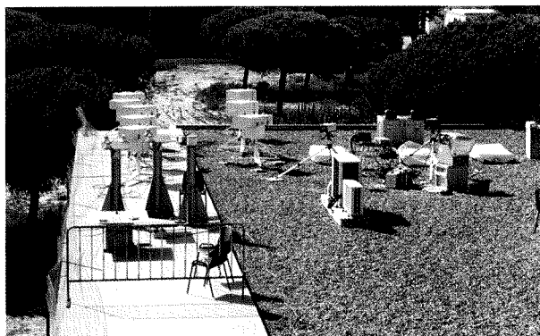
Fig. 1. Instruments location during the blind days, on the left the seven Brewers, on the right the two Bentham over wood boxes, Optronic, Oriel and Licor. The photo was taken from the tower; the main obstacle for the instruments.
