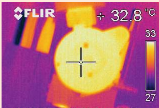
Figure: Temperature of the optical head after temperature stabilization at 32.7 °C
