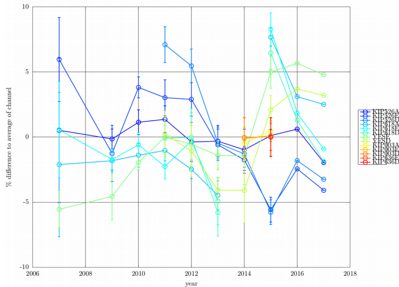
Fig. 1: Variations of absolute calibration factors of ARPA broadband radiometers (the AAO Bentham spectroradiometer was used as reference).
